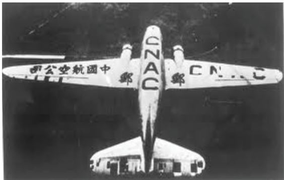
*Note the port wing which is about 5 feet longer than the starboard wing.*
